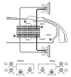
Figure 6. CS50.4 used in bridged 2-channel mode to drive a set of components or subwoofers. Set crossovers according to application.
